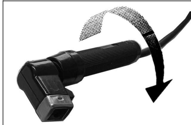
3. Tighten the grip until the electrode is secure.
